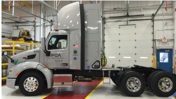
Figure 16. Agility's CNG fuel system installed on FCA Transport truck
